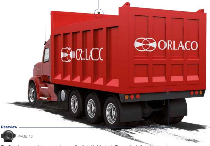
The Rearview camera lets you see the area directly behind the truck. The monitor in the cab automatically switches over to this camera view if you select a reverse gear, allowing you to reverse safely.
