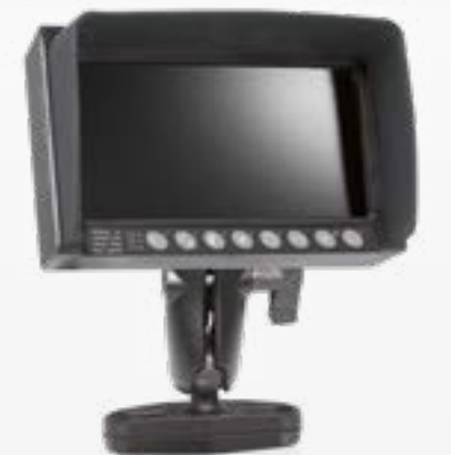
RLED 7" (Incl. User-adjustable 7.5 inch mounting bracket with clamp)
