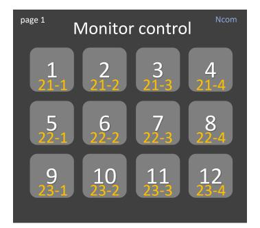
21, 22 and 23 are virtual Unit numbers 1-2-3-4 are virtual Sources. In the App the selected monitor will be controlled by button [5]
